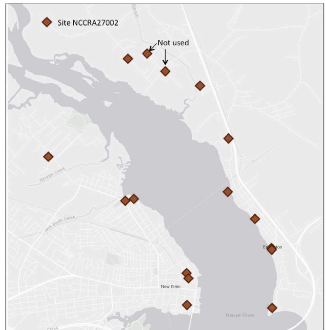
**Fig. 6.** Location of high water marks from Hurricane Florence measured by the U.S. Geological Survey near New Bern used in this study. Data are listed in Table 4, starting at site NCCRA27002 at upper left and moving clockwise to site NCCRA27044.
