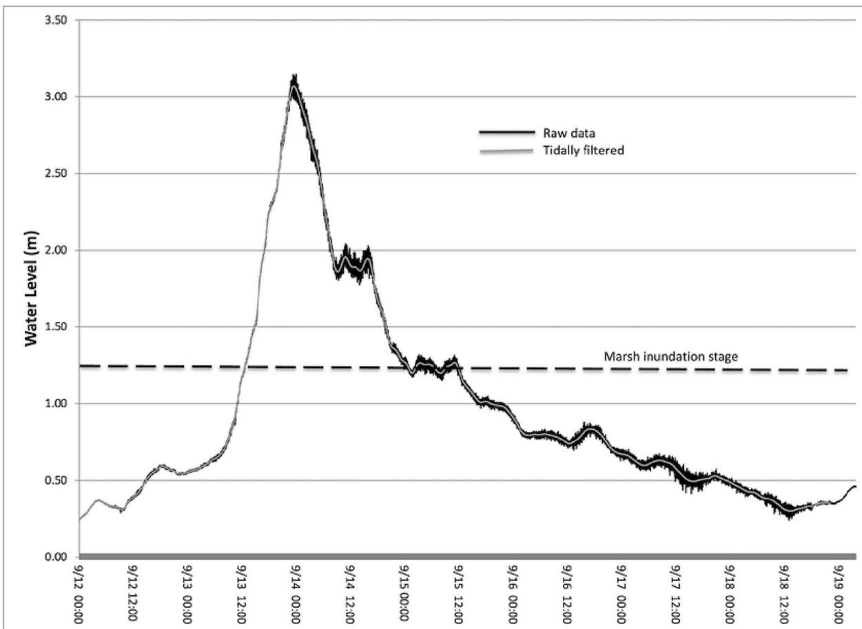
Fig. 7. Water level data from USGS water level sensor NCCRA12508 (see location on Fig. 6) in elevation above mean sea level. The sawtooth line represents unfiltered measurements; the central line is tidally filtered.
